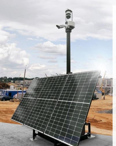
Example Deployment: ARC System (Security Platform) deployed into each corner of the construction site. Each ARC has integrated CCTV Cameras and Radar which constantly sweeping the area and using analytics can detect intruders and alert your monitoring centre. They can issue an audio warning and inform the local security team.
